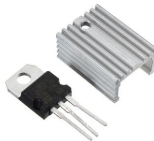
Figure 42 Voltage Regulator IC with Heat Sink
