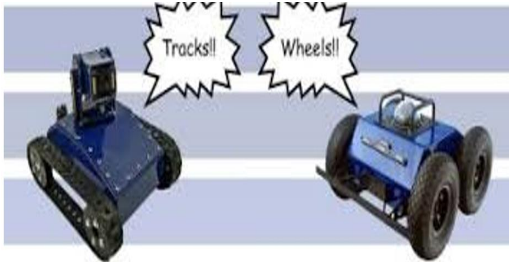
Figure 63 Wheels Vs Tracks
