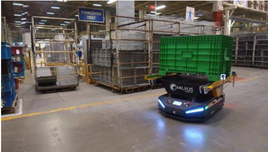
Figure 2: Autonomous mobile robot on factory floor
